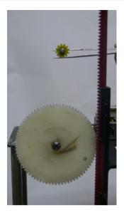
FIGURE 1. Side by side view of the two wheels used for the dip coater. The larger wheel has a radius eight time the smaller wheel, meaning that the larger wheels will result in eight times the velocity of the smaller wheel for any given voltage.
