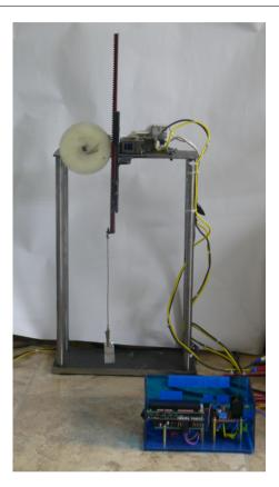
FIGURE 4. Front view of the dip coater with Arduino based microcontroller to the right. The substrate is attached to the alligator clip.
